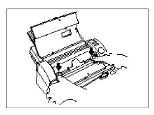
(4) Return the roller holder to the original position and press the roller holder lock buttons (purple color) as illustrated. You will hear the roller holder click into place. Press the roller holder further to secure the roller unit.
